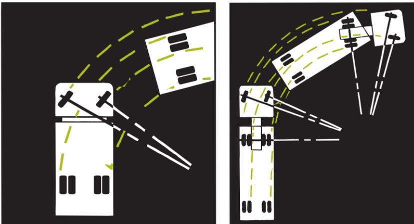
The combination unit of a truck-tractor and “pup” trailer has different turning characteristics than those of the semi-trailer type. These units have turning radius and off-track patterns within each unit, but the amount of off-track is dependent upon the length of the draw bar and the wheel base of the units.
