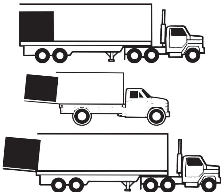
The load should be centred to give the proper wheel load distribution. The average single unit truck has a central weight distribution point midway between the rear of the cab and the tailgate. The average semi-trailer type truck has a central weight distribution point at approximately the middle of the trailer.
